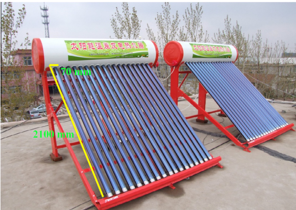
Fig. 6. The pilot STECG co-generator comprised of two evacuated tubular solar collectors, each with 18 tubes. Each tube contains a thermoelectric module.
