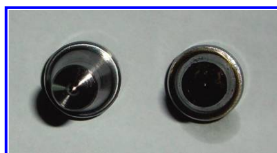
Figure 6. Comparison of injector corrosion using (left) a diesel feed and (right) the OP-ABF/D emulsion.
