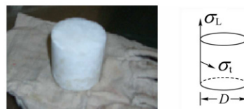
Figure 5. The compaction test sample and the stress analysis
