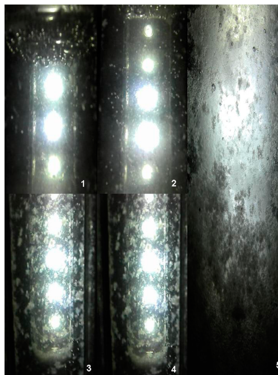
Figure 6. Pictures of the hydrate formation process in the scaled-up equipment at 3.0 MPa and 274.65 K.
