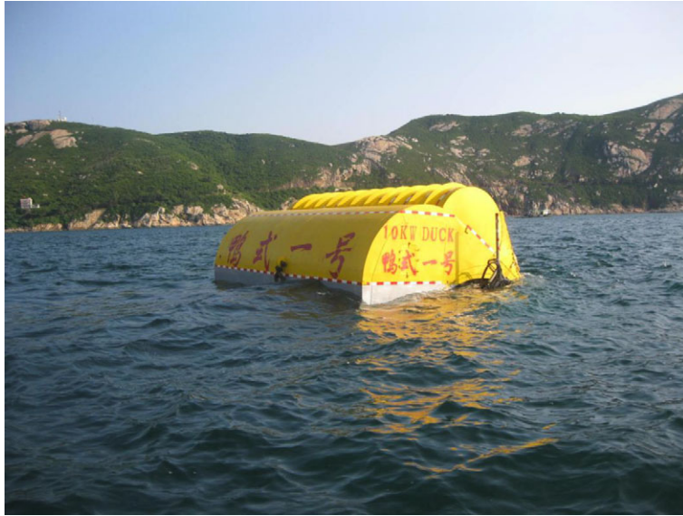
Figure 6. The 10 kW floating Duck in a real sea trial. (Online version in colour.)
